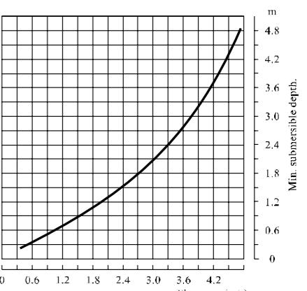
Suggested suction pipe submersible depth vs flow rate
